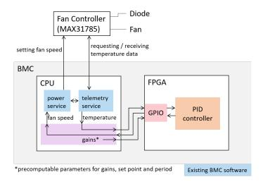
Figure 4: Diagram of the integration of the PID controller into Enzian
