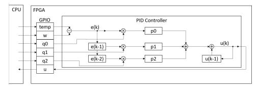
Figure 5: Simplified block diagram of the PID controller
