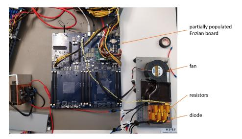
Figure 6: Set up for testing the PID fan controller
