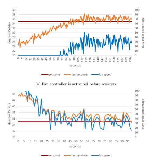
Figure 7: Temperature in  $^{\circ}$ C and fan speed in duty cycle over time
