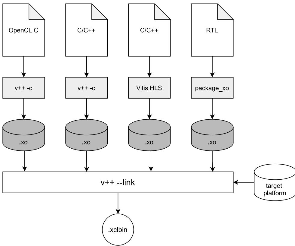
**Figure 2.3:** Vitis device build process
