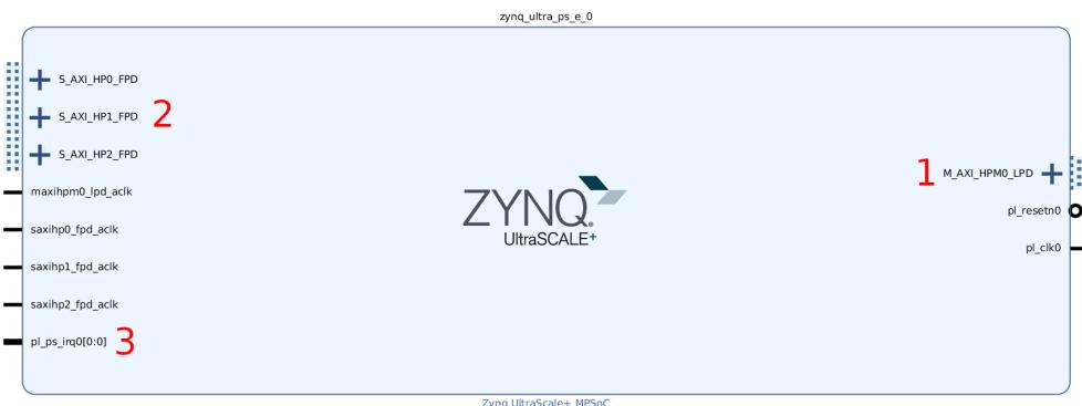
**Figure 3.4:** Processing System IP block
