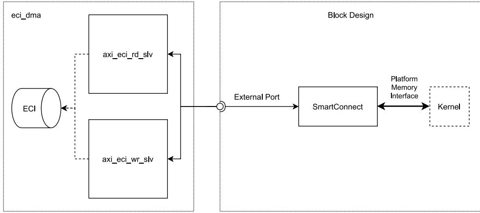
**Figure 3.7:** Path of the memory interface from the CPU to the kernel
