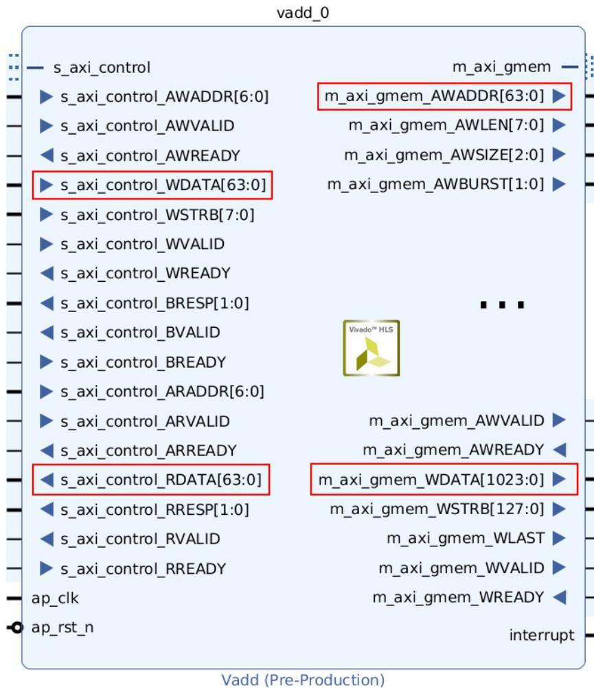
Figure 3.12: vadd kernel IP with correct interfaces
