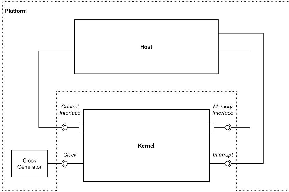
**Figure 3.3:** FPGA design created by the Vitis compiler
