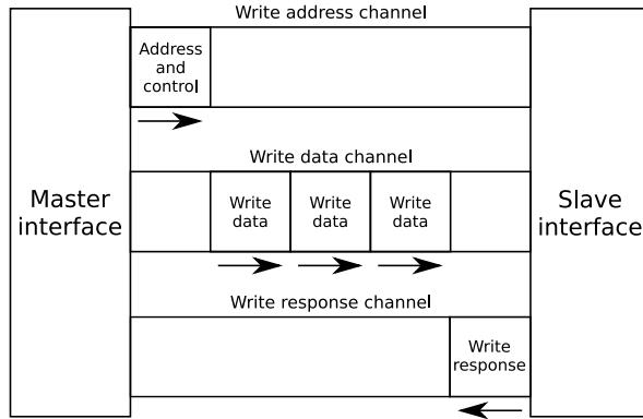
Figure 2.6: AXI write channels [49]
