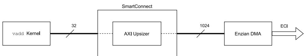
Figure 3.13: Block diagram that illustrates the data width issue
