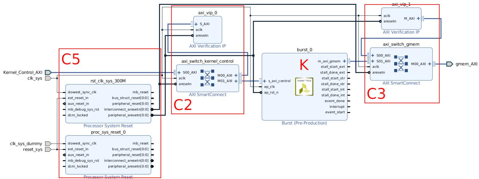
Figure 3.10: Final block design with an example kernel
