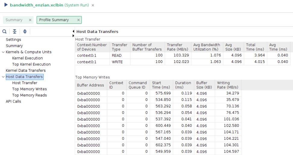
Figure 4.4: Excerpt from a profiling report in the Vitis Analyzer
