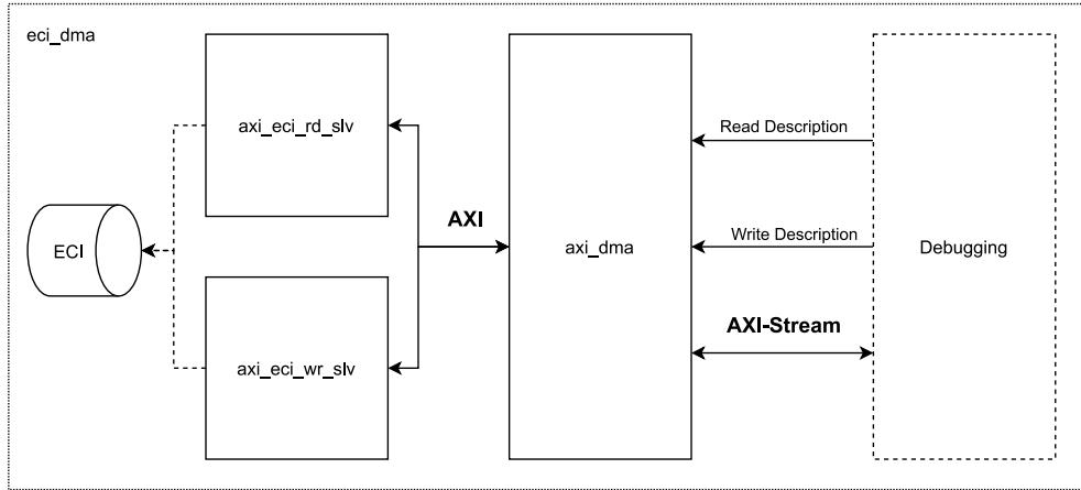
**Figure 3.6:** Enzian DMA architecture
