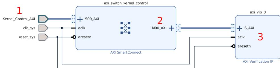
**Figure 3.5:** Kernel control part of the block design
