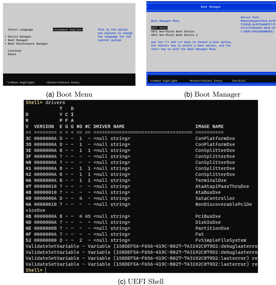
Fig. 4: Terminal interface of the Boot Menu and UEFI Shell
